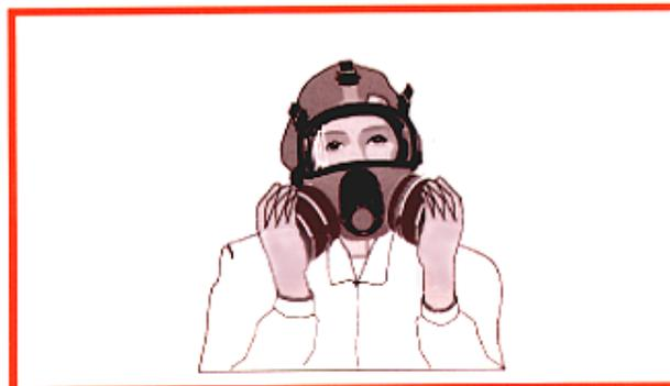
**User Seal Check: worker covering inlet and inhaling
