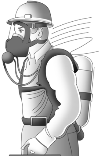
Tight-fitting Self-Contained Breathing Apparatus (SCBA) pressure-demand mode
