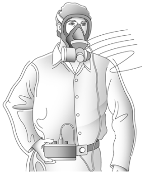
Tight-Fitting Full Facepiece Powered Air-Purifying Respirator (PAPR) APF=1,000 Needs to be fit tested
