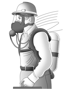
Self-Contained Breathing Apparatus (SCBA) Atmosphere-supplying, or Supplied-air respirator (SAR), which provides clean air from an uncontaminated source Needs to be fit tested APF=10,000
