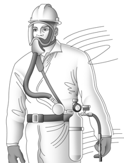
Atmosphere-supplied respirator Full Facepiece Elastomeric with an auxiliary escape bottle APF=10,000 in escape mode only; otherwise APF=1,000 Needs to be fit tested
